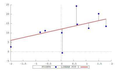
Black segments represent the error we make by substituting  $y_i$  with  $\hat{y}_i$ , that is  $error_i = y_i - \hat{y}_i = y_i - \beta_0 - \beta_1 x_i$ . In this example is  $y_i - \mathbf{6} - 3x_i$ .
